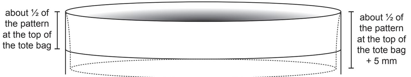
Sew all around, following the line at the bottom border of the printed pattern, using a regular stitch.
